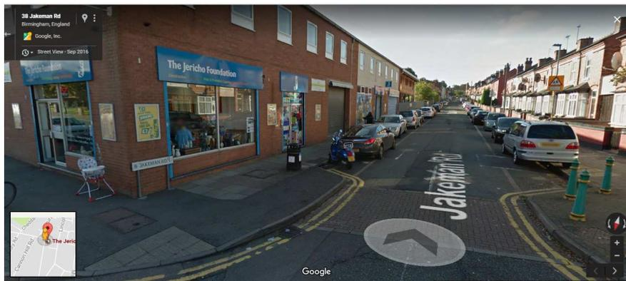
18. Digbeth (CA-02526\_S3\_06\_701): proposal for 8 “M” shaped cycle stands could be made dual use by adding a drop kerb and re-locating pedestrian barrier to inside of the racks with single pedestrian access gap through barrier.
