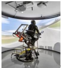
The DESMORI dynamic motorcycle riding simulator has been used for the participant study. It is equipped with a BMW F 800S as mockup, mounted on a six degrees of freedom hydraulic platform. The mockup enables the rider to interact with fully realistic controls, such as a usual handlebar, brake lever / pedal, clutch, gear selector, etc. that he/she is used to. The manual gear shift uses a sequential six-speed gearbox. (photo courtesy of Würzburg Institute for Traffic Sciences).
