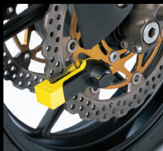
Disc Lock - Use a good one and make sure you make it as inaccessible as possible.
